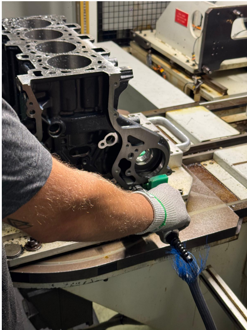
Image 34. Checking the inner diameter of a blind hole in the block with a pneumatic gauging tool, wearing a cut-resistant glove.
