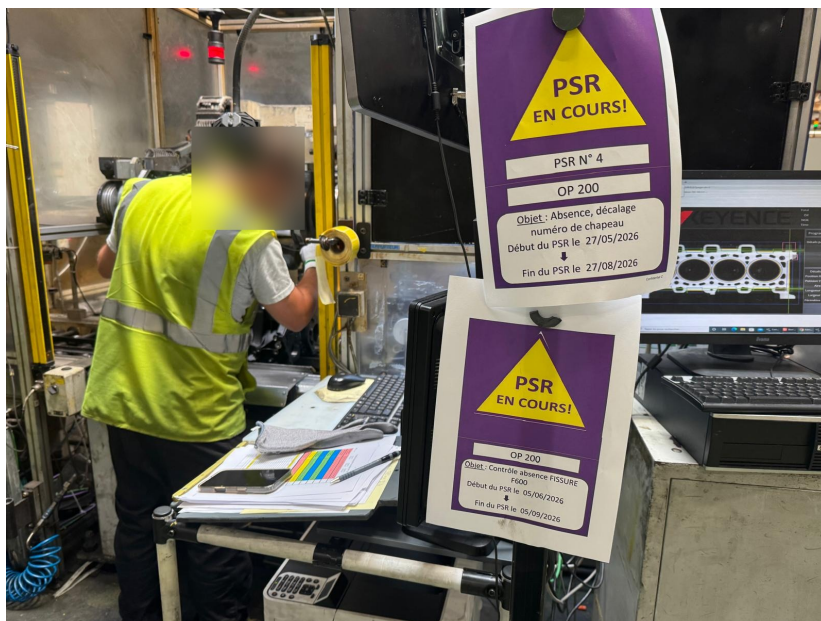
Image 27. Laser scanner inspection station, with two Enhanced Monitoring Plan (PSR) sheets displayed. The first concerns “missing or shifted bearing cap number”: a block’s five bearing caps are numbered 1 to 5 and must be fitted in that order, but on some blocks the order is occasionally reversed, or the number is not visible at all; while this has no effect on engine operation, it still has to be reported to Nissan, who requires it contractually. This defect echoes the bearing cap adjustment described in section 3.5.
