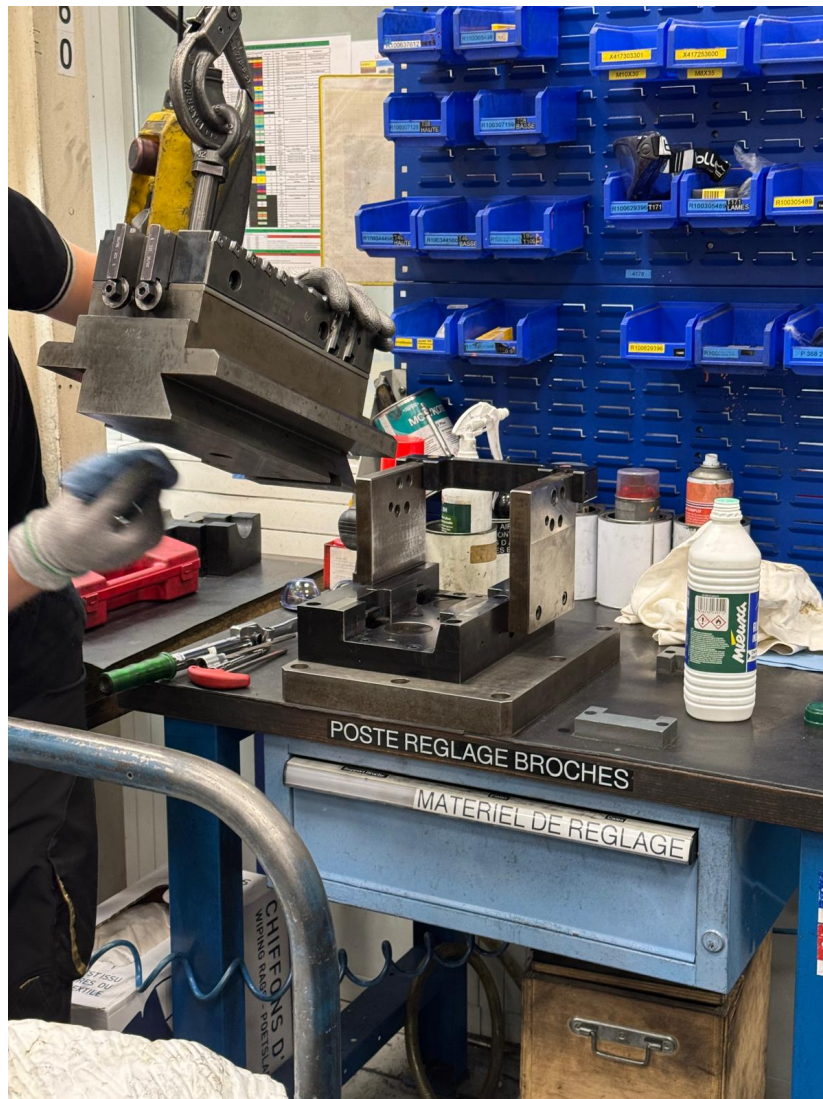
Image 11. The workshop's broach adjustment station: adjusting a precision tool suspended from a hoist, on its reference fixture.
