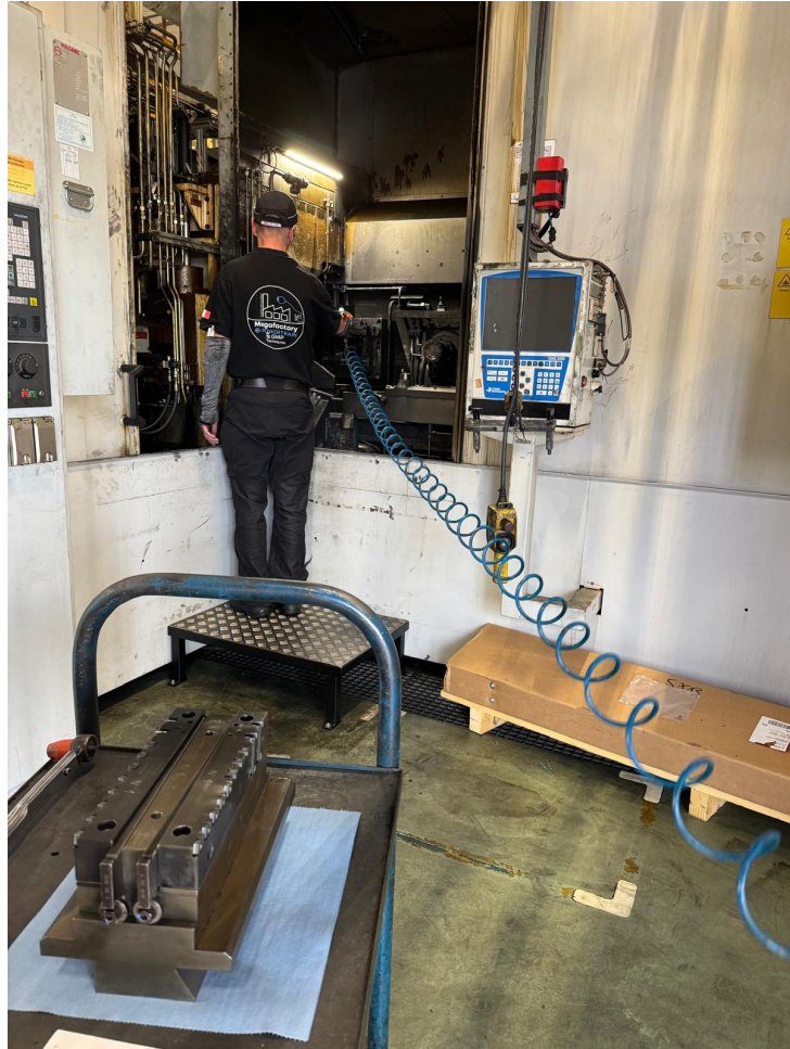
Image 12. [REDACTED], the team leader, adjusting a broach with a high-pressure air blower to remove metal chips and coolant.
