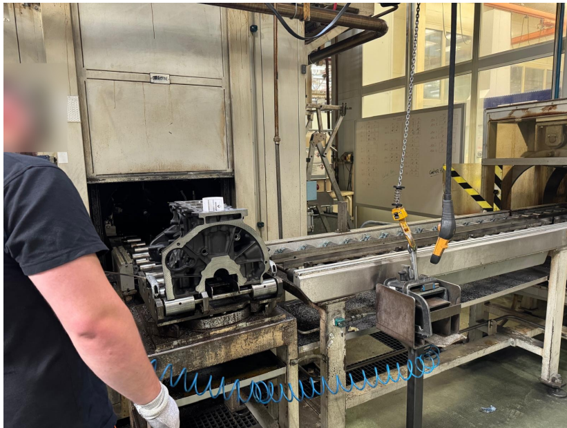
Image 35. Cylinder block coming out of the washing machine: the compressed-air gun's hose (in the foreground) is used to blow off the water before sliding the part onto the conveyor leading directly to the 3D inspection room.
