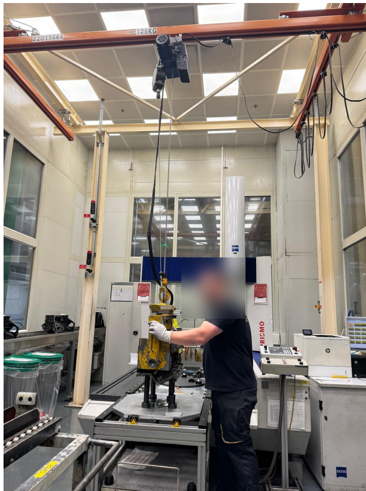
Image 2. Positioning a cylinder block on the fixture of the Zeiss Prismo 3D coordinate measuring machine, using a chain hoist (125 kg capacity).
