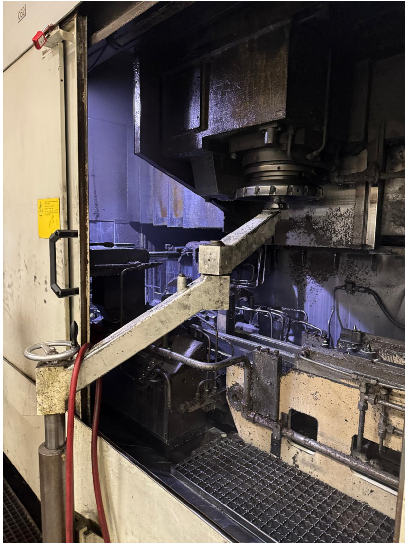
Image 30. Inside one of the workshop's machine tools (cylinders, hydraulic and pneumatic hoses, cable chains), with the lifting arm used to fit and remove the milling cutter: this kind of access requires a lockout padlock to be fitted beforehand.
