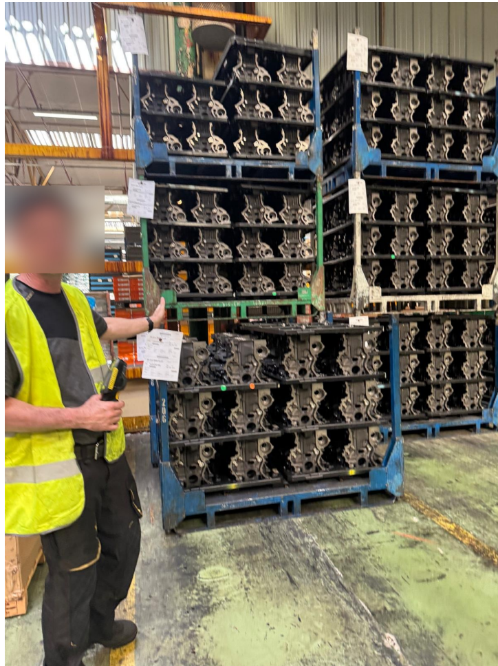
Image 10. A “TM”: a pallet with plastic dividers grouping a batch of inspected blocks, used for storing and moving them around the workshop.
