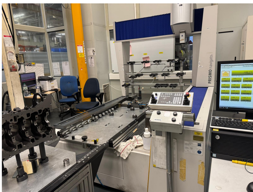
Image 25. 3D coordinate metrology room fitted with the Zeiss Prismo Navigator machine.
