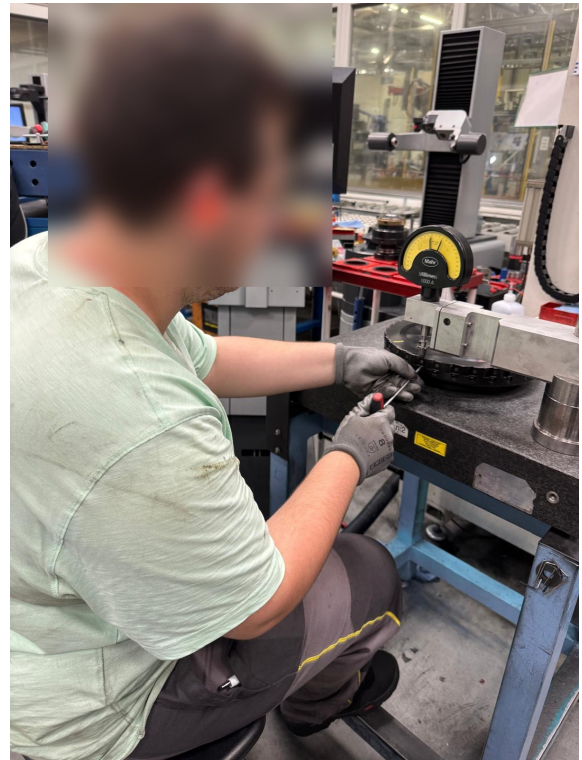
Image 5. Adjusting a milling cutter on the metrology surface plate, using a Mahr Millmess dial gauge.
