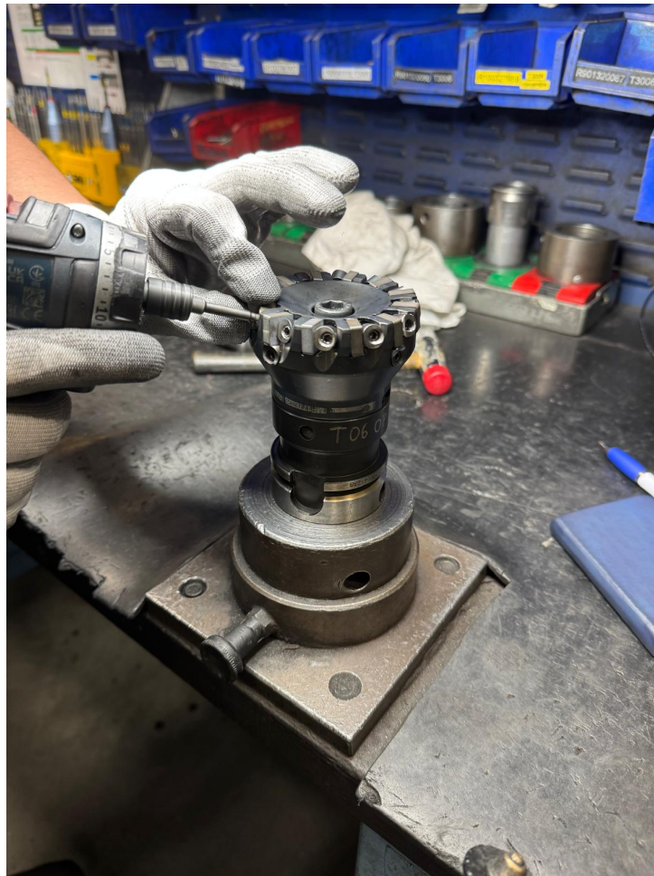
Image 3. Changing a carbide insert on a finishing milling cutter (HSK cone), using a torque screwdriver.
