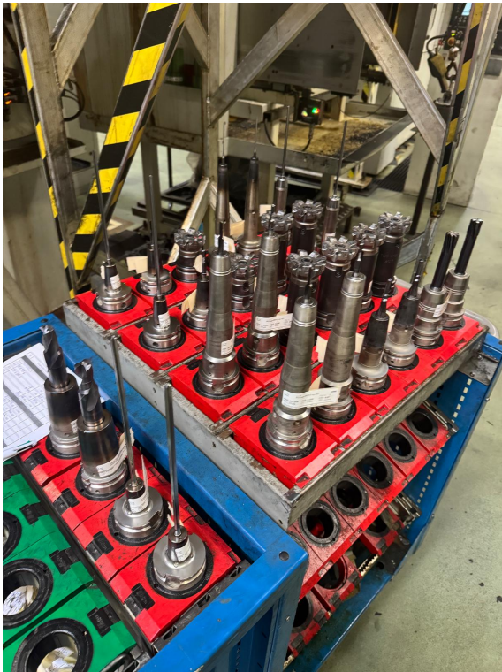
Image 4. Trolley loaded with adjusted milling cutters and drill bits, ready to be refitted at the workshop's stations.
