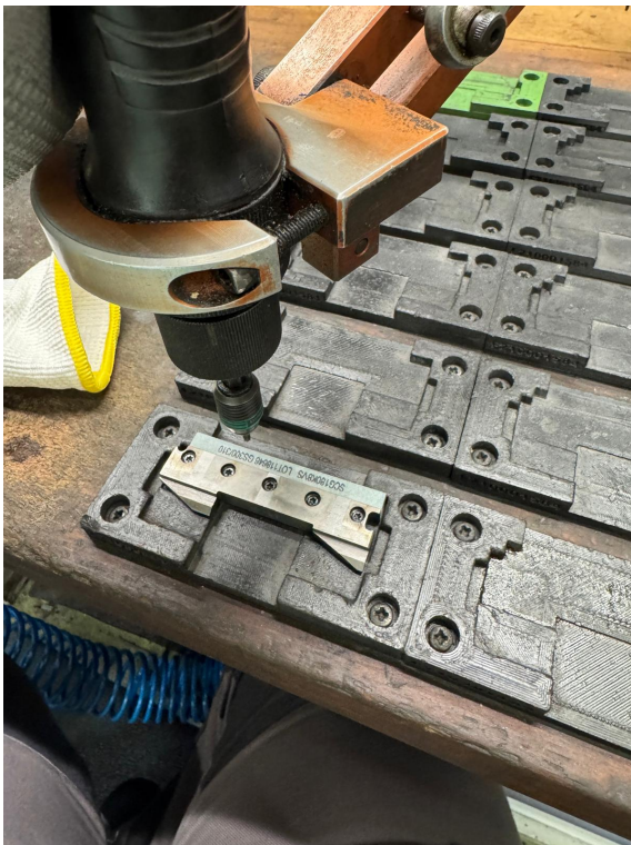
Image 6. Changing a honing stone, mounted in its holder.
