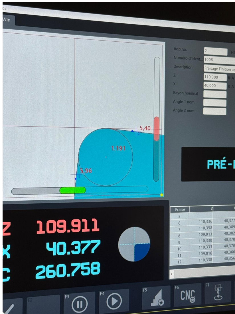
Image 28. Screen of the tool presetting bench (Zoller, pilot 4.0 software): measuring the diameter and position of a finishing milling cutter before refitting.
